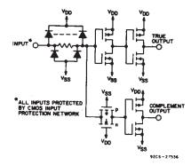
Fig.1 - Schematic diagram 1 of 4 buffers.
