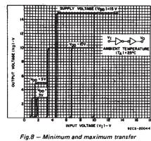
ig.8 — Minimum and maximum transfer characteristics — true output.
